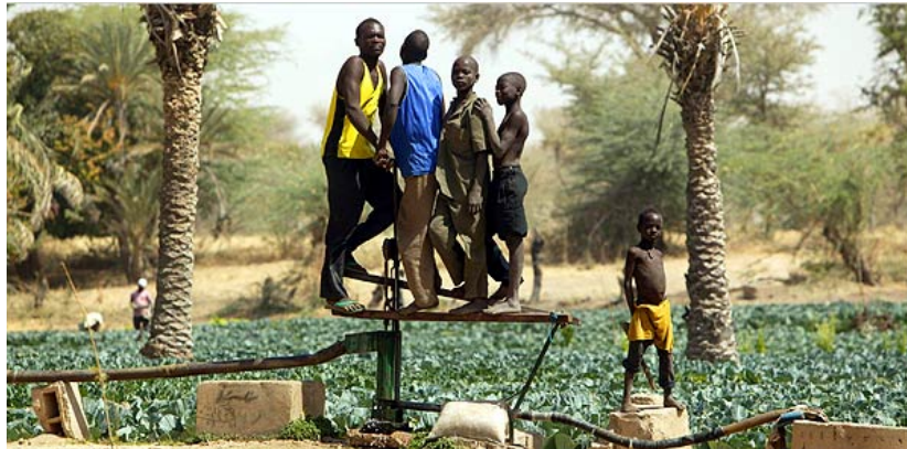
In Ague, Niger, where replanting trees helped alleviate the effects of a famine in 2005, boys operate a foot pump to draw water for irrigation.
