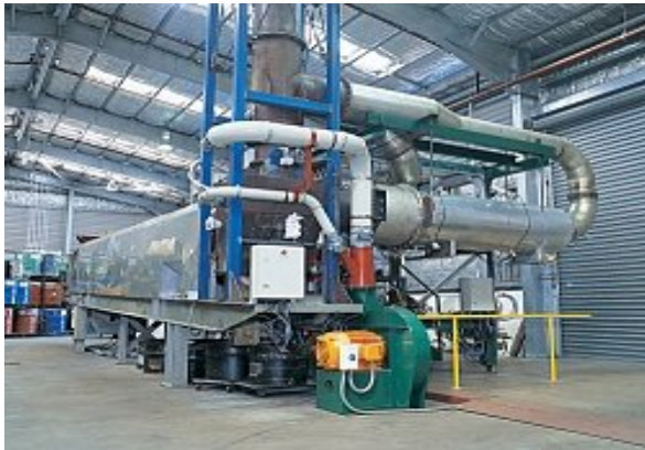
Figure 4. CSIRO-Liquatech 1.2 MW Hybrid Coal and Gas Turbine
